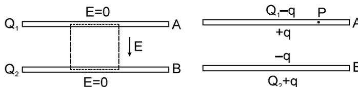
The distribution should be like the one shown in figure. To find the value of  $q$ , consider the field at a point P inside the plate A. Suppose, the surface area of the plate (one side) is  $A$ . Using the equation  $E = \sigma / (2\epsilon_0)$ , the electric field at P
